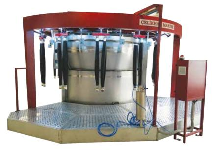
This system has been designed and manufactured to spray on jeans, jackets and shirts, various chemicals such as chlorinederivatives, pigments and resins. It reduces labor costs and increases efficiency
